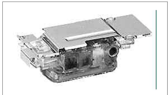
The print head in Canon's Micro BubbleJet Camera has 64 nozzles per color. Source: Canon USA
